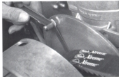
Photo A - Side clearance on the primary pulley can be measured with feeler gauges and should be at least .020 inches for proper de-clutching. Values more than .060 inches can cause slow acceleration.
