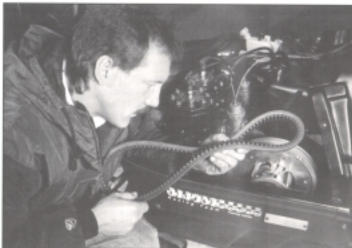
Belt construction is critical as it must slide in and out of the pulleys more than 18,000 times per minute while being squeezed with 2,000 pounds of force.
