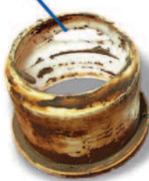
WORN, FAILED BEARING
